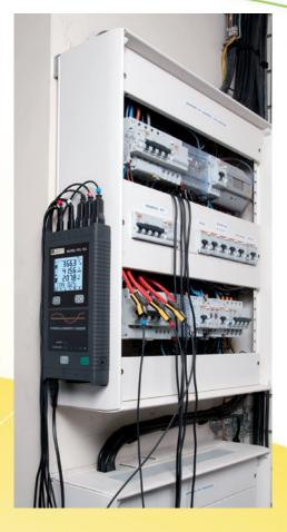
The monitoring by the PEL100 provides the recordings which will be compared with the reference.
